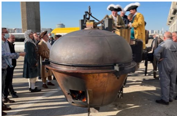
The "Cugnot" – thought to be the first self-powered vehicle. Built in France in 1770. Able to carry four tons, and achieving speeds up to 5 MPH. This steam engine two and a half ton wooden vehicle was spotted and photographed earlier this year at the famous Retromobile car show in Paris by musher Richard Golding,
